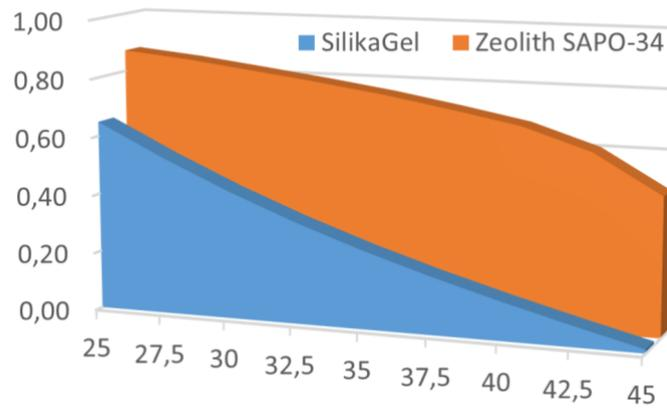
Figure 10: Comparison of Adsorption-potential (kg/kg) of silicate and zeolite in dependency of heat rejection temperatures (x-ordinate), Source: Fahrenheit.
