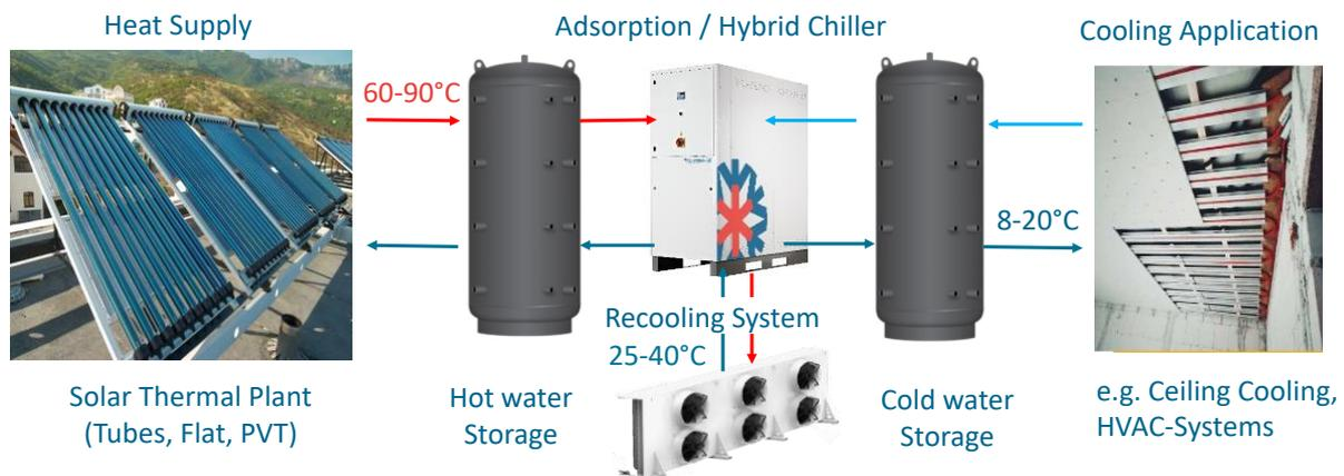
**Figure 9: Typical solar cooling set-up. The system can be run by solar heat up from 60 °C to 90°C and produce cold water with temperatures from 8 °C to 20°C depending on the conditions, Source: Fahrenheit.**
