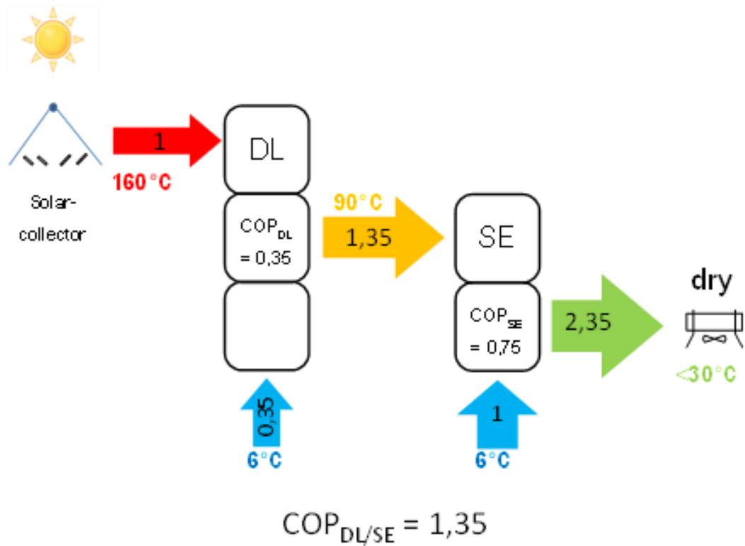
Figure 3: SunBeltChiller combination of double-lift and single-effect chiller, Source: ZAE Bayern.
