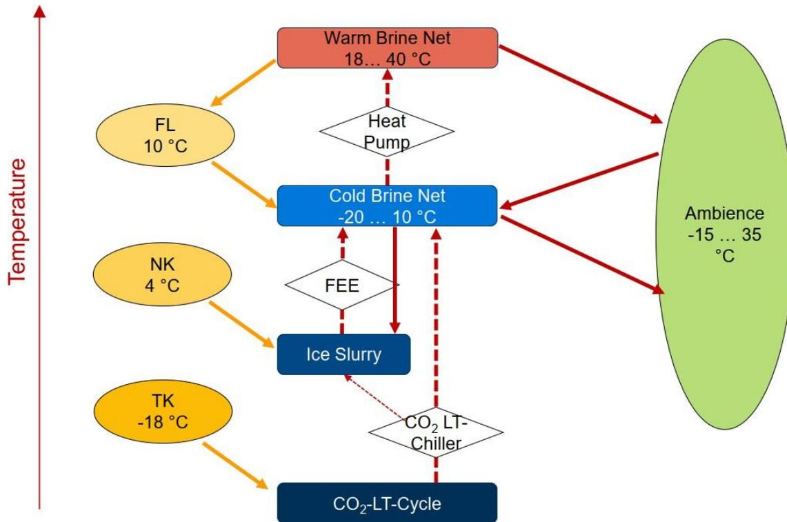
Figure 15: Schematic representation of heat flows, Source: ILK Dresden.
