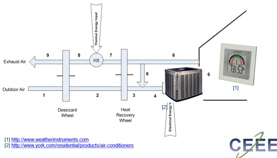
Figure 13: Desiccant and evaporative cooling with PVT collector to regenerate the desiccant system as well as to supply electricity to the vapour compression chiller for sensible cooling, Source: CEEE.
