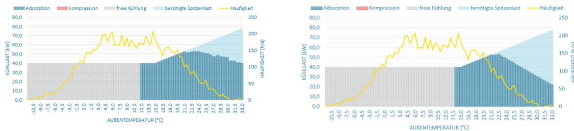
Figure 11: Comparison of dry and adiabatic re-cooling systems, Source: Fahrenheit.
